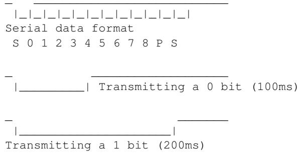
A logical 0 is encoded from the time signal station as a low-level pulse of 100 ms duration and therefore causes the serial controller's input byte to contain binary 11110000 (hexadecimal F0). A logical 1 encoded as a 200 ms low-level pulse simply causes an input byte of 0.
